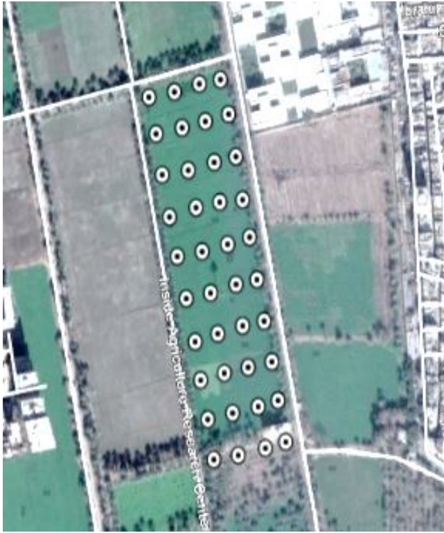
Fig. 1 : Geo-referenced soil resistivity data acquisition grid.
